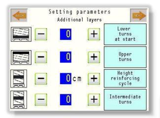
The new user interface by Touch-Screen is highly simple and intuitive and, through this it is possible to manage all operating parameters of the wrapping process.
